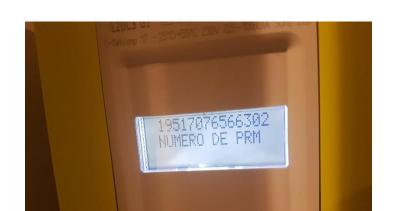
In case of power failure, please check if any breakers has come down. If they are all up, then you just need to push for 4 seconds the "+" button (right button) on the Linky box (pictured)
